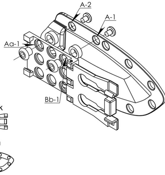
For **HORIZONTAL carry**, screw holes "**A**" and "**Aa**" together, with rubber washers between sheath and Tek-Lok.
